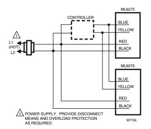
Fig. 11. Common transformer with one controller output and two actuators.
